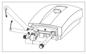
► Use two adjustable wrenches to tighten the middle piece of the hot water union connection.
