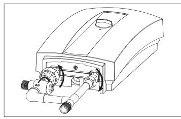
► Hand-tighten the union nuts of the cold & hot water connections on the DHC-E to the corresponding threads on the DHC-E TLC.
