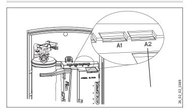
► Connect the lead of the electronic temperature control of the DHC-E to position "A2" in order to get the limit the outlet temperature to 109 °F (43 °C).
