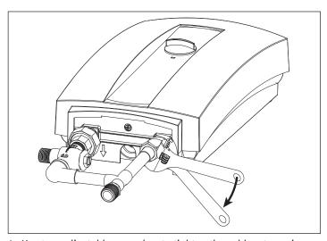
► Use two adjustable wrenches to tighten the cold water union connection by turning the middle piece clockwise.
