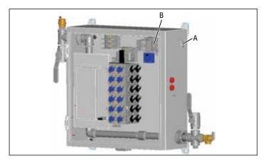
Feed the wire through the knockout (A) using a Romex clamp for strain relief.
