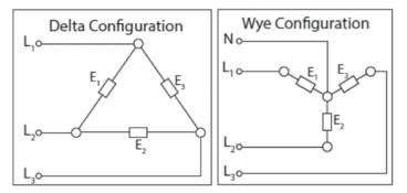
For delta configuration, a three-phase wire and a ground are supplied. For a Wye configuration, a three-phase wire, a neutral, and a ground are supplied. The configuration and voltage are declared on the unit name plate on the enclosure front type plate.
